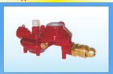
The Two Stage Type 524 AS regulator is mounted directly to tank, connected to the tank valve of ASME container type. It is connected at its outlet to the installation gas pipe net. The regulator inlet POL coupling is equipped with an excess flow valve device.
