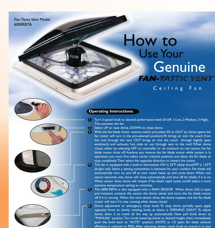
**Recommendations:** You may use your Fan-Tastic Vent while driving or in windy conditions. In this case keep your dome fully open. When storing your Motorhome, lower your dome until it is completely closed and turn the 3 speed knob to 0-Off.
