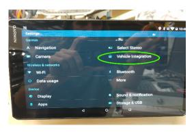
STEP 10. UNDER THE VEHICLE INTEGRATION MENU SELECT STEERING WHEEL CONTROLS (SEE FIG. 10)
