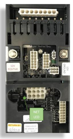
Your G8 panel is the power distribution center for the coach. This panel receives the signals sent from your Spectrum screen/switch panels and performs the actions that have been requested by activating and deactivating the required circuits.
