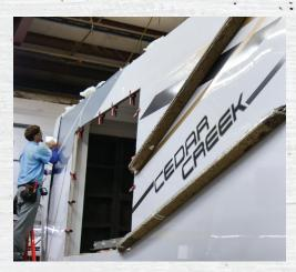
The trailer's strength does not come from the frame, but from the fact that the wall is one piece. Other manufacturers do not build their walls, they just assemble them.
