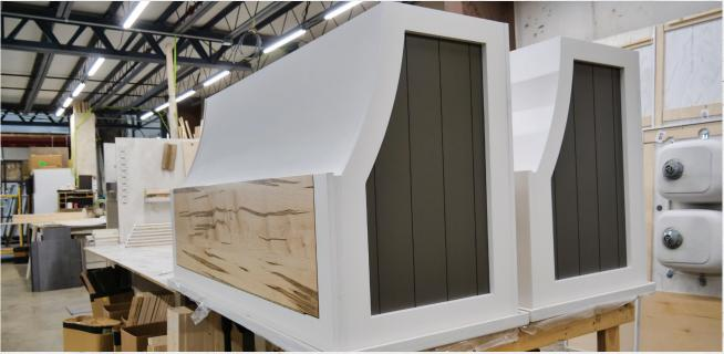
Kitchen cabinets can be one of the most striking features in a new fifth wheel. All of our cabinets are built from quality materials and are hand assembled by in-house skilled craftsmen and women. All lumber core stiles are predrilled and countersunk. This creates long lasting quality cabinetry that will stand the test of time.
