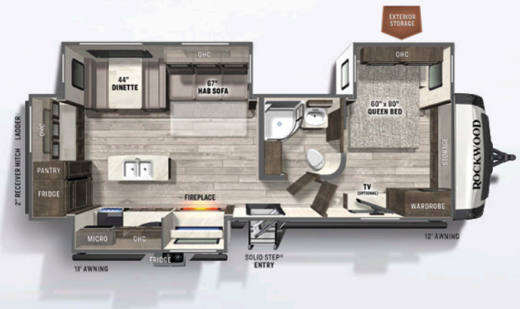
2720IK REAR KITCHEN UVW: 8324 HITCH: 1035 AXLE: 7230 CCC: 1511 LENGTH: 33' 1" ULTRA LITE WIDTH: 8' HEIGHT: 11' 3" FRESH: 54 gal GRAY: 90 gal BLACK: 45 gal
