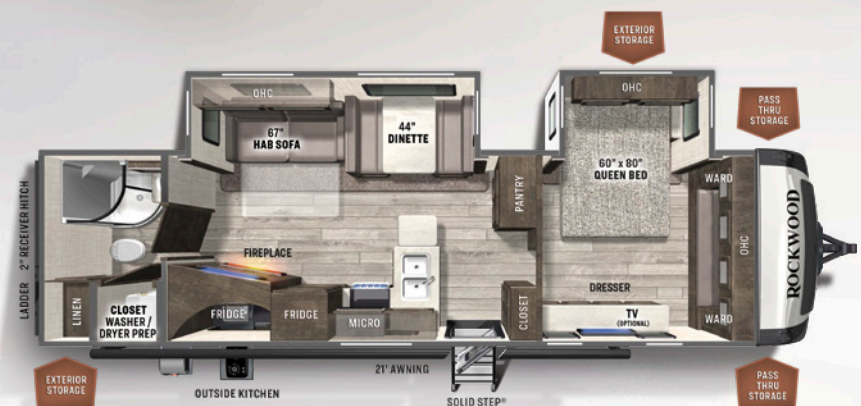
2912BS REAR LIVING UVW: 7854 HITCH: 952 AXLE: 6843 CCC: 1898 LENGTH: 35' 2" ULTRA LITE WIDTH: 8' HEIGHT: 11' 2" FRESH: 54 gal GRAY: 90 gal BLACK: 45 gal
