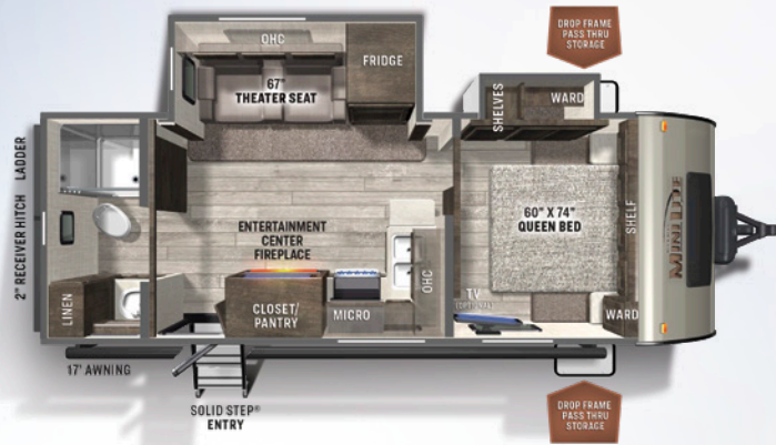
2511S REAR LIVING MINI LITE U/VW: 5492 HITCH: 714 AXLE: 4719 CCC: 1382 LENGTH: 25' 10" WIDTH: 8' HEIGHT: 10' 11" FRESH: 54 gal GRAY: 60 gal BLACK: 30 gal
