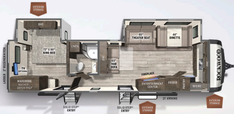
8335SB FRONT KITCHEN SIGNATURE U/VW: 8327 HITCH: 1057 AXLE: 7211 CCC: 2730 LENGTH: 36' 8" WIDTH: 8' HEIGHT: 11' 7" FRESH: 54 gal GRAY: 130 gal BLACK: 50 gal
