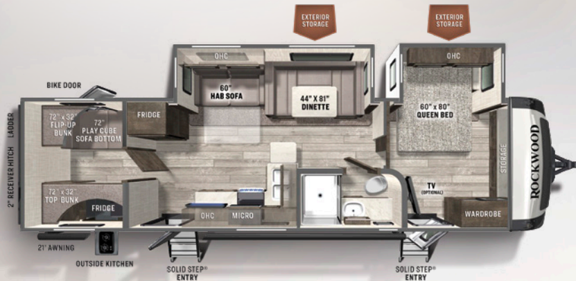
2911SB BUNK HOUSE UVW: 7605 HITCH: 1038 AXLE: 6508 CCC: 2233 LENGTH: 35' 5" ULTRA LITE WIDTH: 8' HEIGHT: 11' 2" FRESH: 54 gal GRAY: 45 gal BLACK: 45 gal
