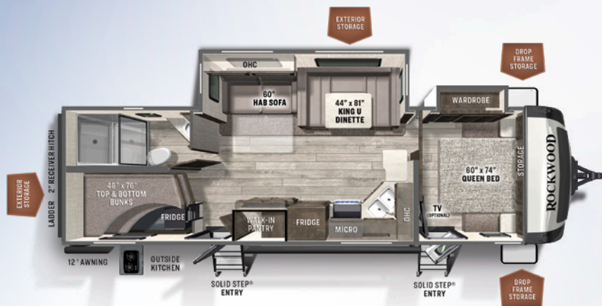
2706WS BUNK HOUSE UVW: 7310 HITCH: 921 AXLE: 6330 CCC: 1411 LENGTH: 32' 10" ULTRA LITE WIDTH: 8' HEIGHT: 11' 2" FRESH: 54 gal GRAY: 90 gal BLACK: 45 gal
