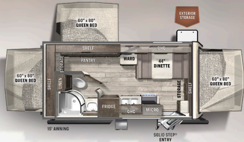
183 EXPANDABLE UUV: 4299 HITCH: 480 AXLE: 3781 LENGTH: 21'2" OPEN LENGTH: 25'7" ROO CCC: 1461 WIDTH: 8' HEIGHT: 10'6" FRESH: 54 gal GRAY: 30 gal BLACK: 30 gal
