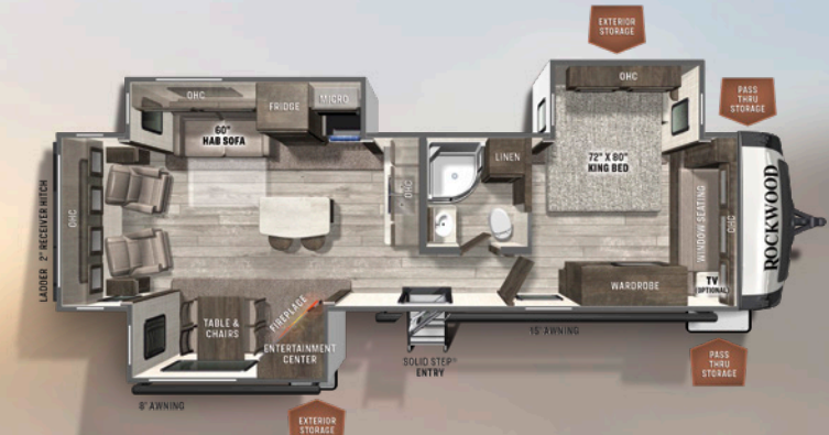
8329SB REAR KITCHEN SIGNATURE U/VW: 8839 HITCH: 1130 AXLE: 7650 CCC: 2291 LENGTH: 36' 8" WIDTH: 8' HEIGHT: 11' 7" FRESH: 54 gal GRAY: 80 gal BLACK: 50 gal
