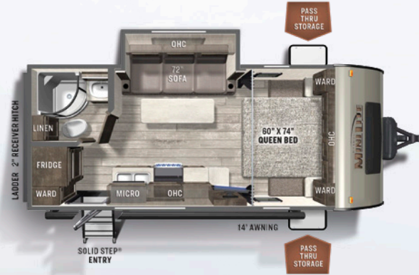
2109S REAR LIVING UVW: 4171 HITCH: 412 AXLE: 3700 CCC: 1521 LENGTH: 22' 4" MINI LITE WIDTH: 8' HEIGHT: 10' 3" FRESH: 54 gal GRAY: 30 gal BLACK: 30 gal
