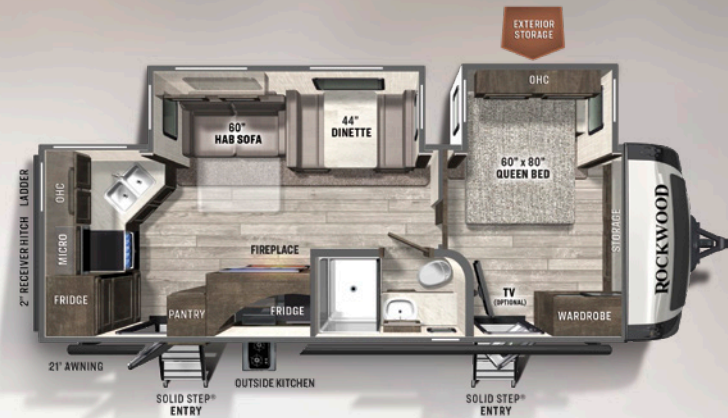
2614BS REAR KITCHEN UVW: 6988 HITCH: 796 AXLE: 6133 CCC: 1608 LENGTH: 29' 9" ULTRA LITE WIDTH: 8' HEIGHT: 11' 2" FRESH: 54 gal GRAY: 90 gal BLACK: 45 gal
