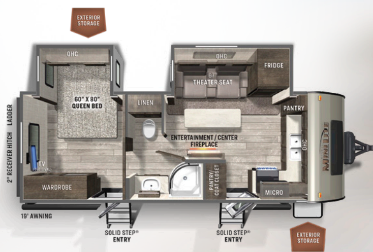
2516S FRONT KITCHEN MINI LITE U/VW: 6033 HITCH: 810 AXLE: 5164 CCC: 1777 LENGTH: 25' 11" WIDTH: 8' HEIGHT: 10' 11" FRESH: 54 gal GRAY: 60 gal BLACK: 30 gal
