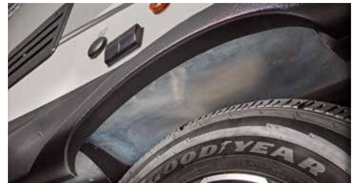
Galvanized Steel, Impact-Resistant Wheel Wells
