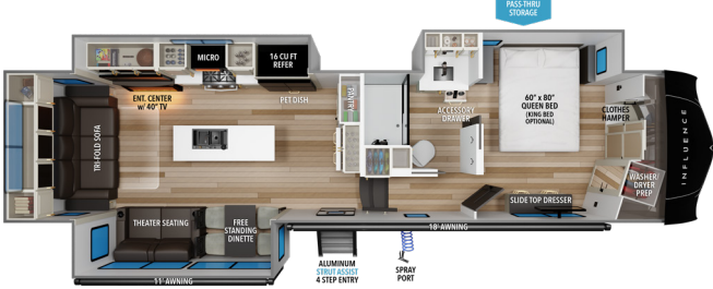
3503GK UVW 1 13,500 HITCH 1 2,670 GVWR 18,000 LENGTH 2 38' 3" HEIGHT 3 13' 5" CAPACITY 83 106 53
