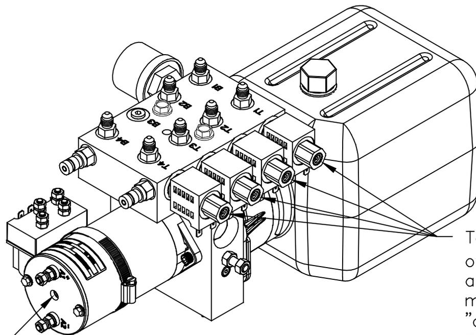
Manual override screw, 6mm allen head, is under this sticker. Using a 2000 rpm minimum drill, retract jacks by turning counter clockwise. To extend, turn screw clockwise.
