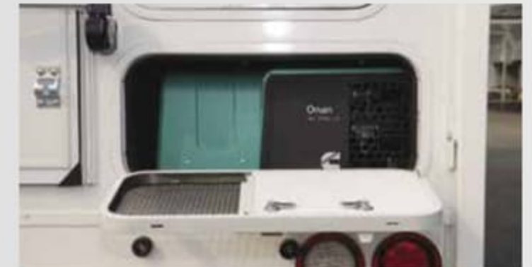
All new Onan 2500W Generator that features an ultra-quiet design. - 855s, 960, 975, 995, 1062, 1172
