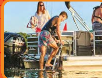
Rear boarding platform w/4-step telescoping boarding ladder & grab rails
