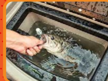
Aft rotomolded compartment w/8-gal. (30.28 L) aerated livewell
