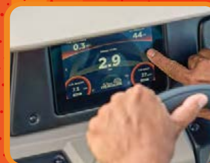
NEW SUN TRACKER FLARE™ touchscreen gauge display & 12-button switch panel
