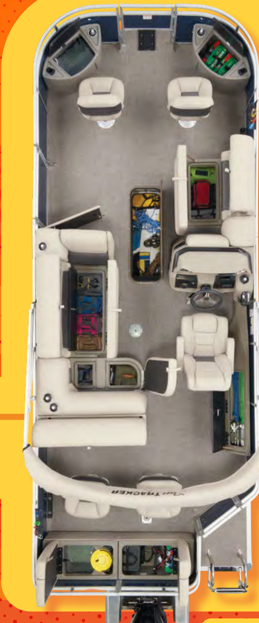
Aft fishing station 16-gal. aerated livewell w/removable bait bucket & shutoff valve
