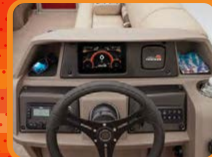
Driver console w/ SUN TRACKER FLARE™ touchscreen gauge display & 12-button switch panel
