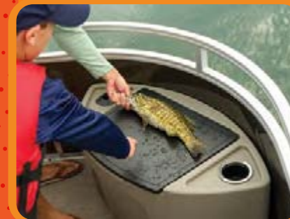
Bow 16-gal. aerated livewell/baitwell w/shutoff valve, drink holder, rod holder & lid w/fish ruler
