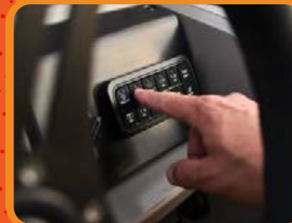
NEW driver console w/integrated storage & 12-button switch panel
