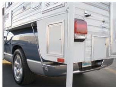
The 815's optional add-on short bed modification skirts make the 815 compatible with short bed full-size trucks, provide extra storage, and the required brake and tail lights.
