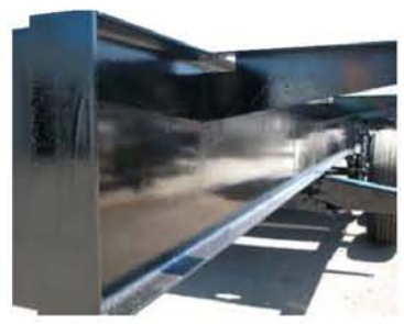
Heavy Gauge Structural Steel I-Beam Main Rail
