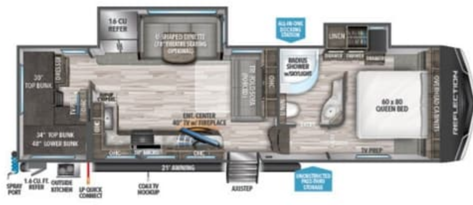
28BH UVW 1 9,198 HITCH 1 1,696 LENGTH 2 34' 8" HEIGHT 3 12' 3" CAPACITY 74 86 43
