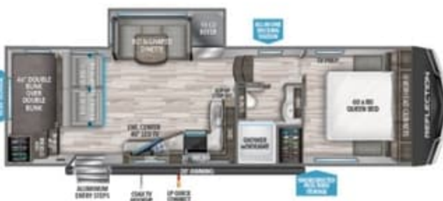
268BH UVW 1 7,893 HITCH 1 1,268 LENGTH 1 31' 11" HEIGHT 1 12' 0" CAPACITY 56 71 39
