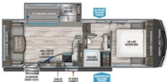
260RD UVW 1 7,534 HITCH 1 1,269 LENGTH 1 29' 9" HEIGHT 1 12' 0" CAPACITY 56 71 39
