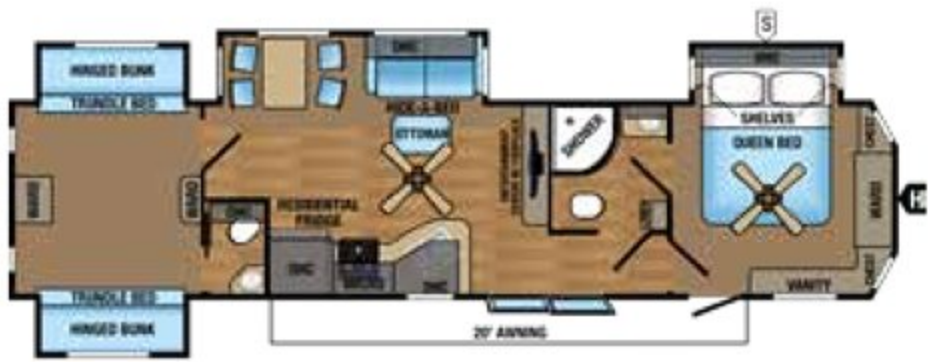
JAY FLIGHT BUNGALOW | 40BHQS OPTIONS: A, B, C, D Ext. Lgth: 40' 2" Ext. Ht: 151" Unloaded Wt (lbs.): 11,220 Sleeps: 6-10
