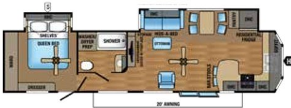
JAY FLIGHT BUNGALOW | 40FKDS OPTIONS: C, D Ext. Lgth: 40' 11" Ext. Ht: 152" Unloaded Wt (lbs.): 10,425 Sleeps: 2-4
