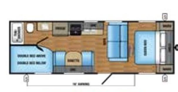
JAY FLIGHT SLX | 264BHW Ext. Lgth: 29' 3" Ext. Ht: 126" Unloaded Wt (lbs.): 4,615 Sleeps: 8-10
