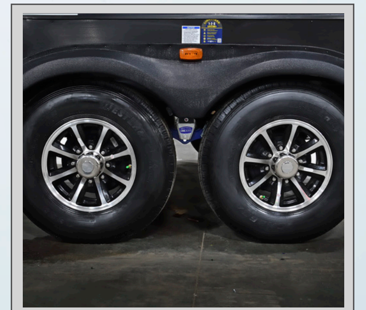
NITROGEN FILLED G-RANGE TIRES 14-Ply Nitrogen Filled G-Range Tires Rated for 4,080 LBS Each
