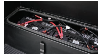
Two batteries in a single housing for easy access. (One battery in LE and Transit)
