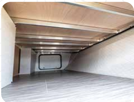
WELDED ALUMINUM BED FRAMING (16/19 SERIES ONLY)
