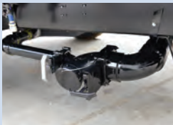
Pivoting Sewer Head for Easy Positioning and Better Ground Clearance
