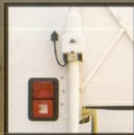
Optional Electric Jacks make loading and unloading your truck camper quick and easy.
