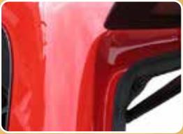
**Specialized Rain Gutters** direct rainwaters and snow melt to keep seals secure and cargo dry.
