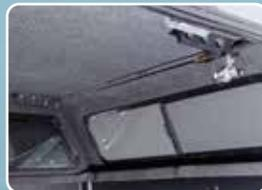
**Sportsman Package** dials up cap strength to support loads up to 500 pounds thanks to its double-reinforced one-inch thick roof. Package also includes four fishing rod holders.
