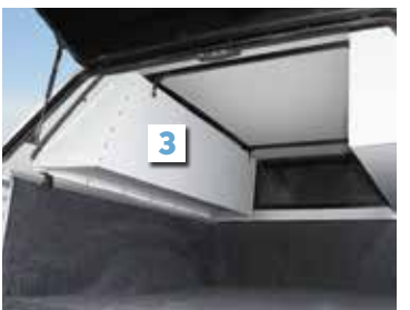
Toolboxes are securely fastened to roof framework
