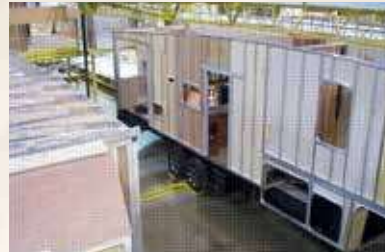
Cedar Creek's famous residential All-aluminum Super-structure (Roof, sidewalls, and floor) on 16" centers or less.
