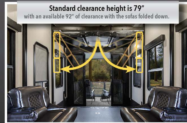
Happi-Jac electric bunk system with folding sofas provides maximum headroom in the garage area. (398M shown)
