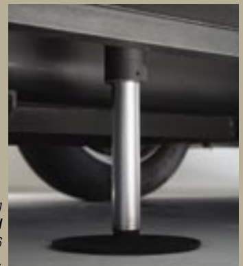
Automatic hydraulic leveling jacks (both extend and retract) are new for 2006 and very easy to operate.
