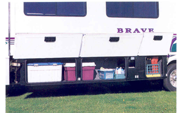
35C Our StoreMore™ Hydraulic Slideout System takes the pain out of accessing storage bays. The spacious compartments extend with the room, so you don't have to crawl under the slideout to get to your gear.
