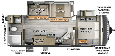
2606WS LENGTH: 29' 9" WIDTH: 8' HEIGHT: 11' 2" HITCH: 840 AXLE: 5742 UWW: 6641 CCC: 1999 F 54 GAL G 90 GAL B 45 GAL
