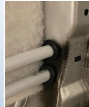
Plumbing lines that pass-through chassis steel are rubber grommets to protect the integrity of the system and prevent future wear issues.
