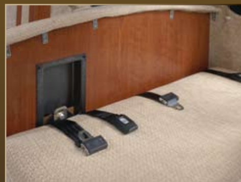
Tether anchor behind booth dinette cushion securely holds child's safety seat while traveling.
