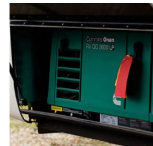
Generator – 3.6 KW LP c/w Auto Start and Auto Changeover Switch
