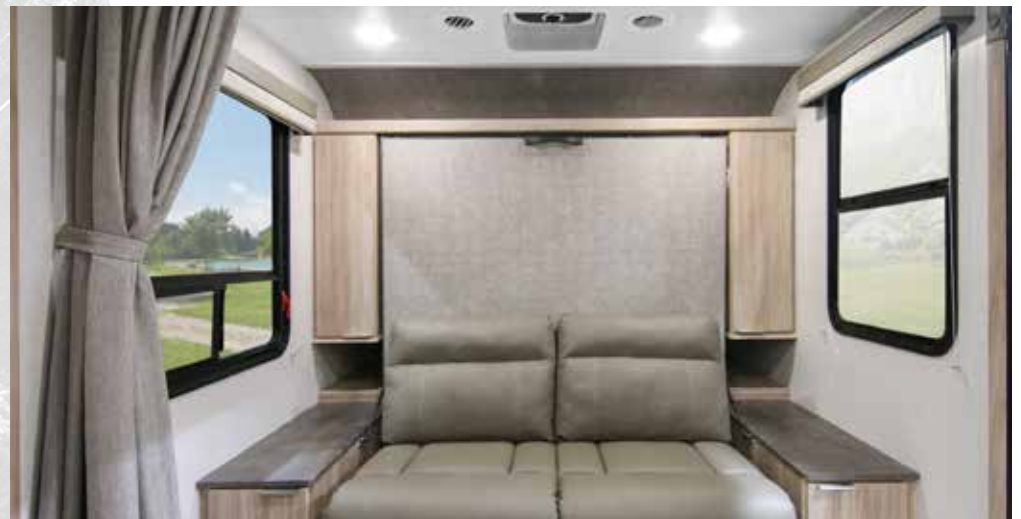
The redesigned murphy bed in the 2108DS floorplan allows the bed to easily fold up and out of the way.
