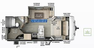
LENGTH: 25' 11" WIDTH: 8' HEIGHT: 10' 11" HITCH: 773 AXLE: 4667 **25**BRDS UVW: 5499 CCC: 1434 6 54 GAL 6 29 GAL 8 29 GAL
