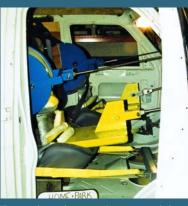
These 2 photos depict simultaneous seat belt pull testing and seating system testing. Seat belt testing confirms proper seat belt location and minimizes the possibility of anchorage failures. Seating system testing verifies the integrity of the seats, their attachments, mounting hardware and installation.
