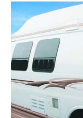
Frameless awning windows are better looking, reduce wind noise, improve aerodynamics, and provide superior air circulation even during foul weather. Their larger size provides a better view from inside. The Integrated Venting System (170 and 190 models) provides inconspicuous ventilation of the refrigerator.
