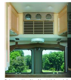
The heat pump (air conditioner & heater) with ducts to the front and rear bed areas is mounted outside of Chevy based Roadtreks for easy service access and external water drainage.
