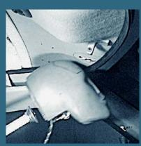
Occupant head protection testing is intended to ensure occupants have additional head protection from interior components during crashes.
