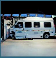
For frontal impact testing, the test vehicle impacted a fixed barrier at 30-mph (48 km/h). Again our test vehicle did not leak any fuel.
