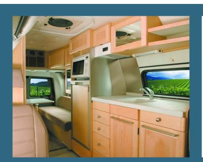
The expanded galley has a larger window and a longer and deeper counter. A toast & bake microwave oven and 4 cu.ft. refrigerator are located after the galley to create more space for 5 deep drawers and a huge cupboard below the counter. The twin beds are wider (30") and the king bed is wider as well (6'8").
