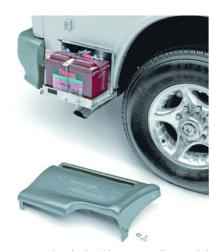
A large capacity auxiliary lead acid battery is totally concealed yet easily accessible on slide-out tray. A second auxiliary battery is optional on 190 and 210 models.
