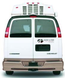
A 'Dometic' heat pump (air conditioner & heater) built into a recess in the roof cools the interior while maintaining Chevy based Roadtrek's aerodynamic shape and sleek roofline. In many restricted communities, vehicles with roof mounted air conditioning units are not permitted. Our recessed heat pump allows our Chevy based motorhome to be perceived as just a van and in most cases is permitted to park where many other motorhomes are not.
