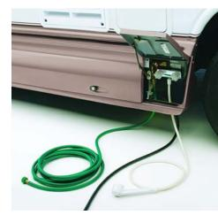
There is a separate compartment for an exterior shower and city water connection with quick disconnect. The 210 features a detachable power cord for trips away from the campsite.
