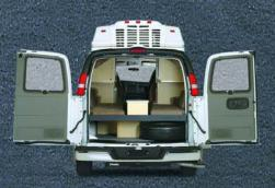
Dual rear doors allow for easy rear loading and swing a full 180° on 170 and 190 models and 270° on RS models.
