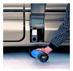
Easily accessible, our patented built-in sewage hose system on 170 and 190 models provides a permanently attached sewage hose that eliminates messy handling and storage. The wastewater tank releases and the fresh water tank drain are adjacent.
