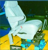
Seating system testing minimizes the possibility of failure of the seats, their attachments and their installation.
