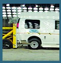
This photo shows the rear impact test. The test vehicle was impacted by a moving barrier at 30-mph (48 km/h). The entire fuel system was then inspected for leakage. Our test vehicle did not leak any fuel.
