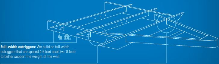
**Norco® NextGen frame:** White Hawk features the industry's best strength-to-weight ratio thanks to a Norco NextGen frame made of high-strength, low-alloy sheet steel, Huck® bolts and an interlocking design.
