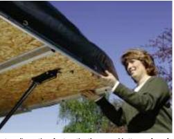
"Weyerhaeuser agrees with Fleetwood's practice of not coating the exposed bottom surface of the Structurwood® panels used in their trailers. In our opinion, moisture from occupancy load, or from other internal or external sources may become trapped in the Structurwood® substrate if it is coated on the underside with a system that impairs the ability of the substrate to dry thoroughly. Trapped moisture, over time, may cause premature decay or rot." Weyerhaeuser
