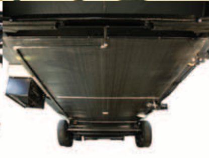
Enclosed underbelly protects trailer components as well as increasing aerodynamics
