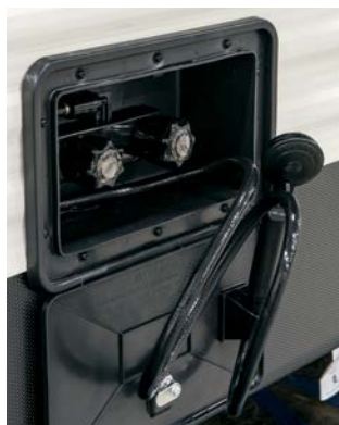
OUTSIDE SHOWER with hot and cold faucets.
