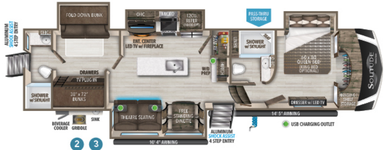
3950BH U/VW 1 HITCH 1 GVWR LENGTH 1 HEIGHT CAPACITY 3950BH-R 14,054 2,584 16,800 40' 4" 13' 5" 91 100 106
