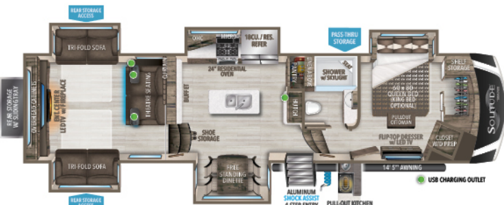
375RES U/VW 1 HITCH 1 GVWR LENGTH 1 HEIGHT CAPACITY 375RES-R 14,200 2,900 16,800 41' 4" 13' 5" 93 100 50
