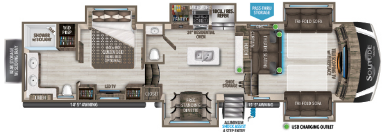
380FL U/VW 1 HITCH 1 GVWR LENGTH 1 HEIGHT CAPACITY 380FL-R 14,866 3,052 16,800 41' 5" 13' 5" 93 106 106
